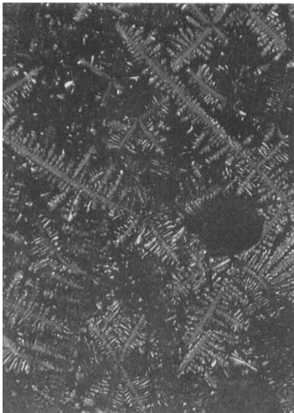
Figure 4. The optical texture observed through the polarizing microscope on cooling 6j to 25°C from the isotropic liquid.
